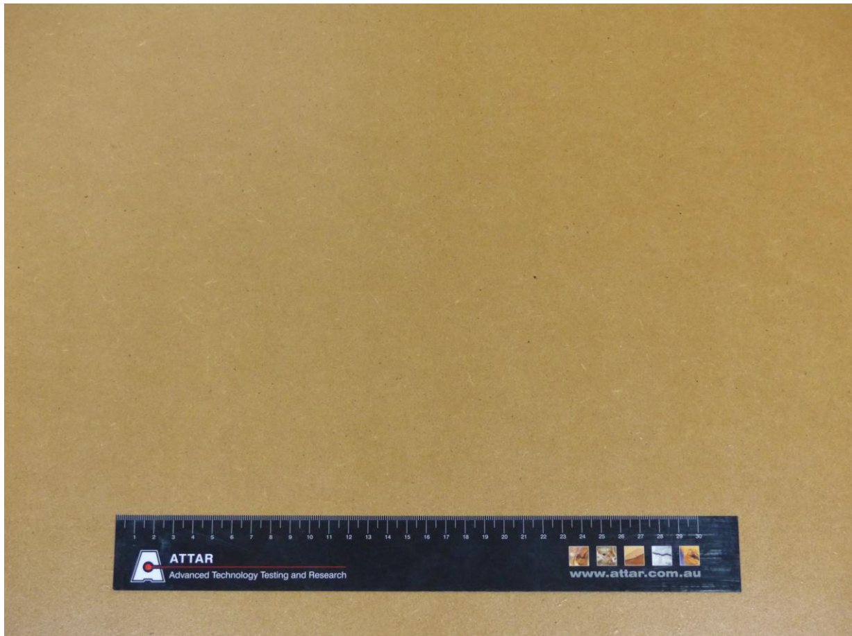
Figure 1: Coating applied to MDF board, coating consisting of one coat Cabot's CFP Oil Based Gloss, One coat Cabot's CFP Oil Based Gloss with 5% Intergrain Ultragrip added, One coat Cabot's CFP Oil Based Gloss.
